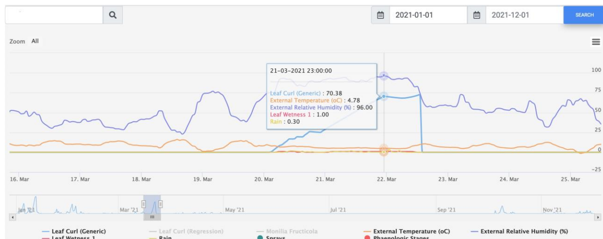
Figure 13. Visualisation of pest infestation risk index along with related data from sensors 39 .
